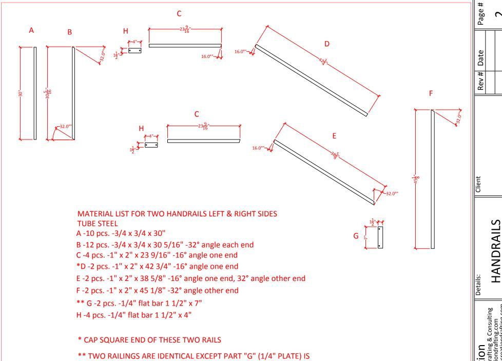
WELDED TO OPPOSITE FACES TO ALLOW MOUNTING TO EACH SIDE OF STAIRS
